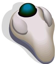
It reminds of a mouse that is lying up side down. The ball usually has about 3 cm in diameter and at least two keys. Such solutions is not a good alternative for a big part of disabled persons – moving a small ball of the trackball is usually more difficult than mowing whole mouse. There are also tools projected with the view of disabled users such us Roller Plus Trackball. Very effective are also trackballs for children. They usually have bigger ball, for example BIGtrack.
